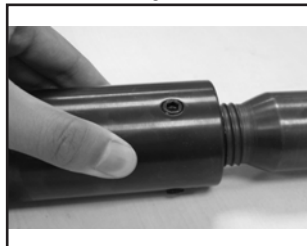
Fasten Needle Scaler to Air Hammer.
